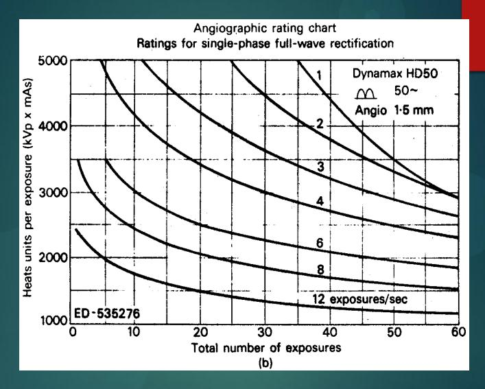
An exposure factors of 100 kV, 300 mA and 0.05 sec generate 1500 HU
